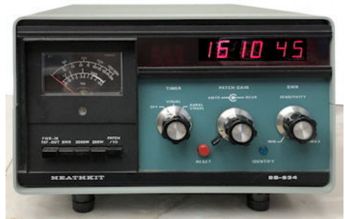
FIGURE 1: The Heathkit SB-634 Station Console. A combination SWR Meter, Dual Range RF Power Meter, Ten Minute Timer and Phone Patch.
