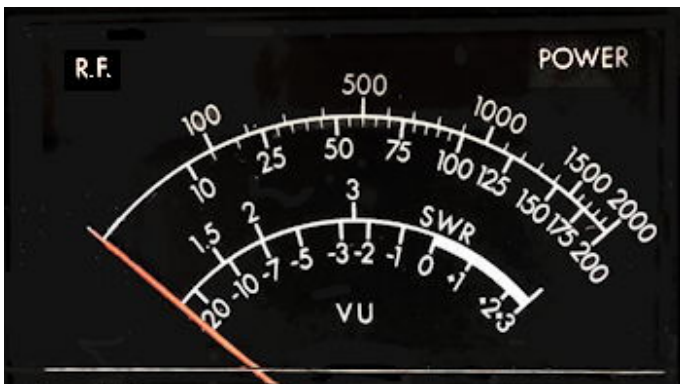
FIGURE 2: Heathkit SB-634 Meter reads Power (0–200 or 2K watts), SWR, and Phone Patch VU. The meter is not illuminated.
