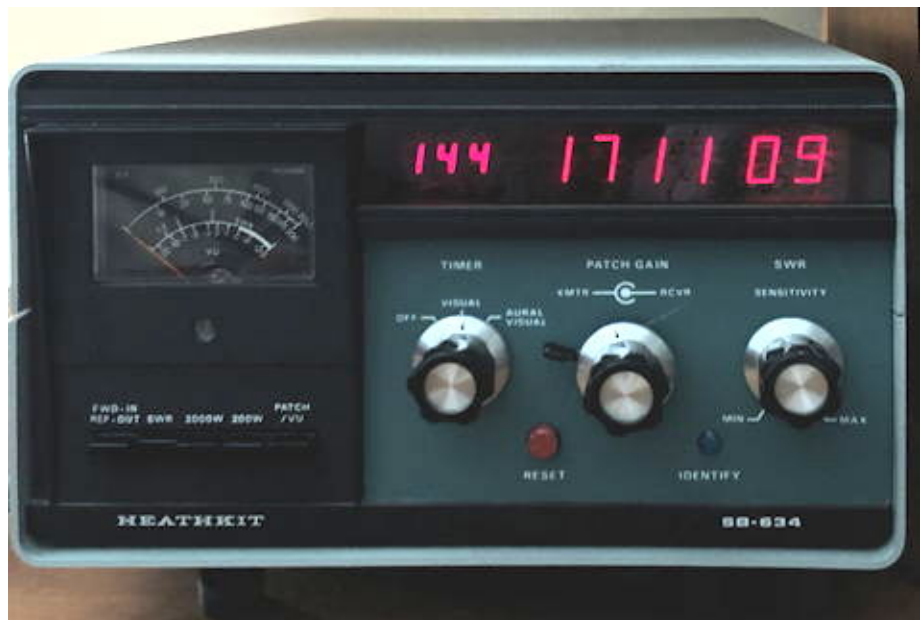
Figure 6: Heathkit SB-634 showing smaller timer digits left of the time digits. 144 (1 minute 44 seconds into the 10 minute period.)
